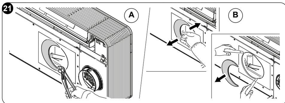
The rear cover is also prepared for the rectangular intake channel. If this type of installation is preferred, break the rectangular precut and use an intake grille of a size suitable for the intake channel.
